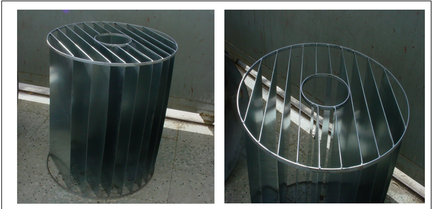
Photo A2.4: Side and top view of the filter before adding RPF (Reticulated Polyurethane foam)
